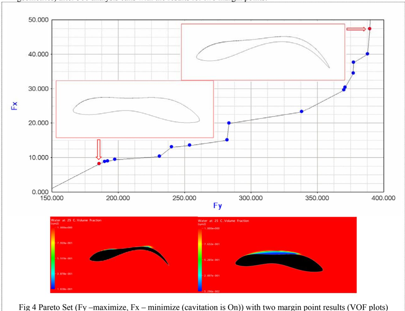
Fig 4 Pareto Set ( $F_y$  –maximize,  $F_x$  – minimize (cavitation is On)) with two margin point results (VOF plots)
