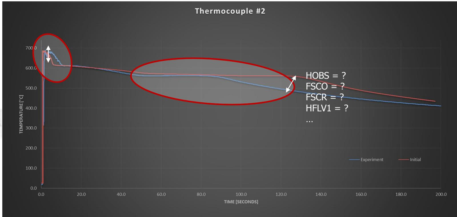
The goal of this study is to optimize numerical parameters to set in **FLOW-3D** to match both the filling dynamic and the solidification behavior.
